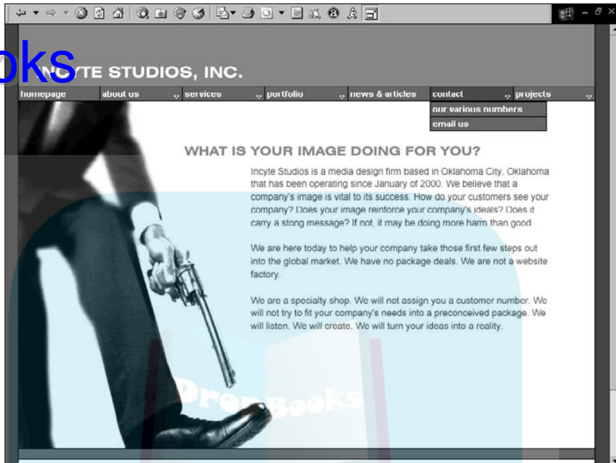
Figure 7-7: This entire page is invisible to search engines. It's made up of one large image and a JavaScript navigation tool.
